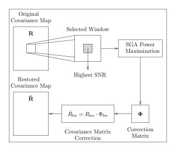
Fig. 4. Proposed phase calibration method.
