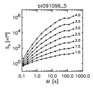
**Fig. 5.** The structure function of the magnetic field shown in Fig. 2. Curves are labeled with the power q.
