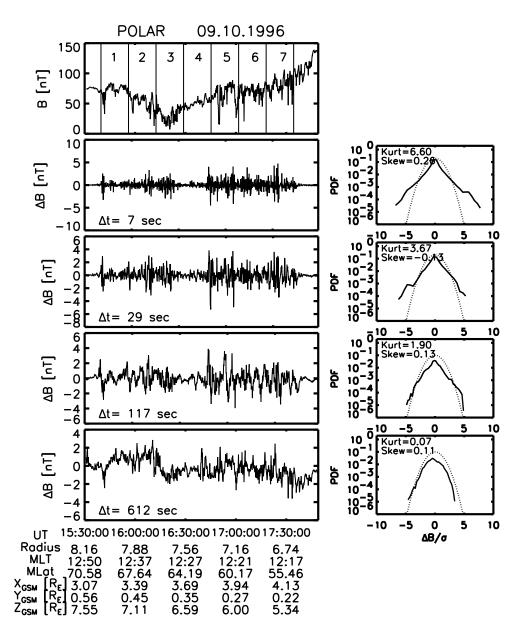
**Fig. 1.** Total magnetic field B (upper panel) and differences  $\Delta B(t) = B(t + \Delta t) - B(t)$ . Right plots show the probability distribution function of  $\Delta B$  normalized to its standard deviation. The dotted curve represents the equivalent Gaussian distribution. Kurtosis and skewness are also given. The data segments used in the analysis are marked with vertical lines in the upper panel.
