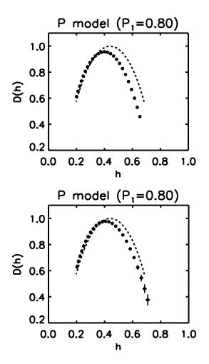
**Fig. 6.** Singularity spectra of the *p*-model calculated directly from the wavelet transform modulus maxima (upper) and by the Legendre transform (lower). Errors were calculated and are shown only for the Legendre transform method. Dashed curves represent the theoretical singularity spectrum.
