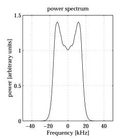
**Fig. 2.** Synthetic data used for the simulations. Pseudo-random white noise was passed through a filter made from an analytical spectrum. The panel to the left shows a 20-ms section of the data, while the panel to the right shows a power spectrum estimate from 10 s of data.
