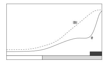
**Fig. 1.** Sketch of the changes observed in the magnetic field and electrostatic potential during the crossing of a quasi-perpendicular shock (based upon the experimental results of Eselevich et al. (1971)).
