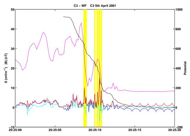
**Fig. 7.** The magnitude (red), and  $E_x$  (blue) and  $E_y$  (cyan) components of the spin plane electric field measured by Cluster 3 on 5 April 2001 around 20:25 UT. The yellow regions highlight the periods when large amplitude short duration spikes in the electric field are observed. The black line (Y scale of RHS) represents the change in potential within the shock.
