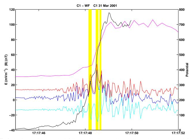
**Fig. 4.** The FGM magnetic and EFW electric fields measured by Cluster 1 on 31 March 2001 around 17:18 UT. The magnetic field magnitude is shown by the magenta line. The spin plane electric field magnitude , and  $E_x$  and  $E_y$  components are shown in red, blue and cyan, respectively. The yellow regions highlight the periods when large amplitude short duration spikes in the electric field are observed. The black line (Y scale of RHS) represents the change in potential within the shock.
