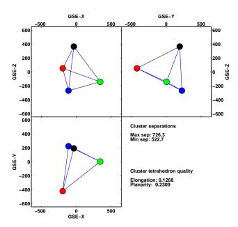
**Fig. 2.** The configuration of the Cluster tetrahedron as they encountered the shock on 31 March 2001 at 17:18 UT. The different satellites are shown using the colour scheme black, red, green, and blue for satellites 1, 2, 3, and 4, respectively. This colour scheme is used throughout this paper when multi-satellite data are plotted.
