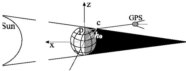
**Fig. 1.** Scheme for the determination of the shadow altitude  $h_0$  over the ground in the GSE system. GPS – GPS navigation satellite; P – GPS station on the ground; C – intersection point of the transmitter – receiver LOS and the shadow boundary.
