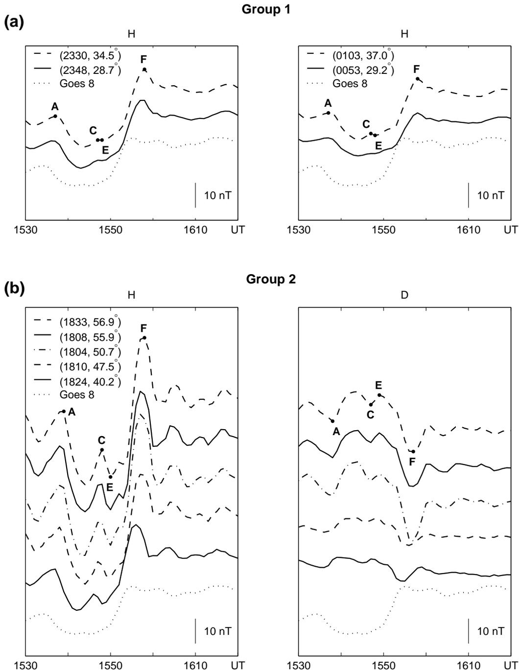
**Fig. 3.** (a) The magnetic field observations ( $H$  component) for two different MLT sectors in group 1. (b) The magnetic field observations for a single MLT strip in group 2. Left plot:  $H$  component, right plot:  $D$  component. In the bottom trace of each panel the magnetospheric field from Goes 8.
