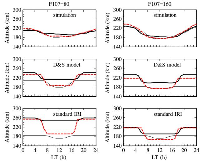
**Fig. 4.** Seasonal effect shown by the simulated LTH and the IRI model (standard IRI and D&S model) at two solar activity levels: left panel for  $F107=80$ , and right panel for  $F107=160$ . Heavy solid lines for summer, dash lines for equinox, and light solid lines for winter.
