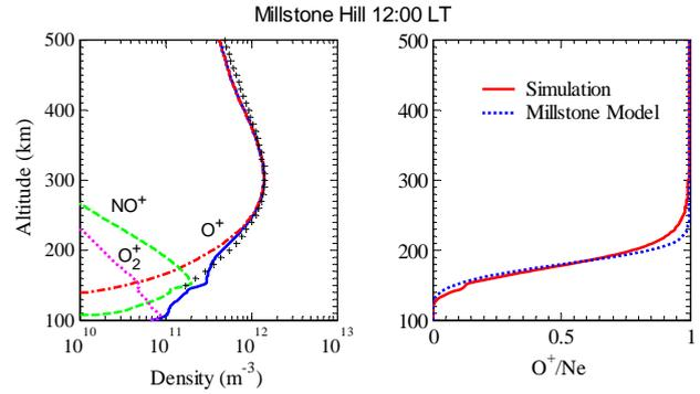
**Fig. 2.** Example of the comparison between the observed electron profile (symbol “+”) and the model (solid line) on 27 September 2000, and  $O^+$ ,  $O_2^+$ , and  $NO^+$  concentrations are also presented (left panel). In right panel, calculated  $O^+/Ne$  are compared to the Millstone Hill standard ion-composition model.
