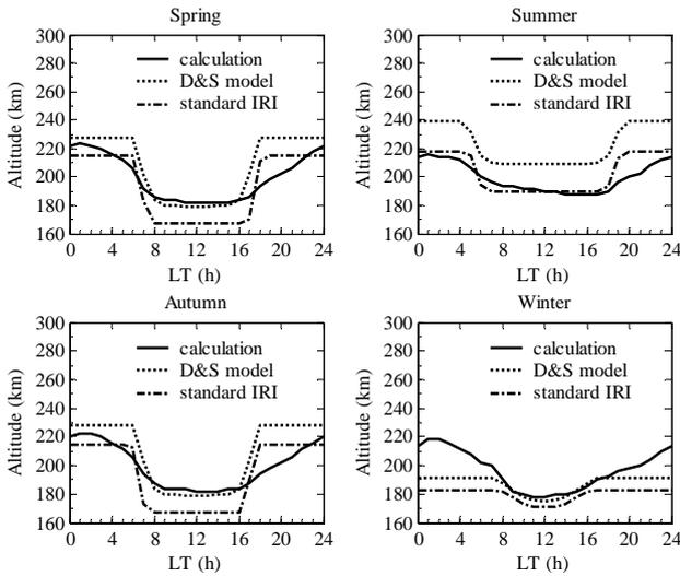
**Fig. 3.** Diurnal variation of the lower transition height as given by the simulated results, the standard IRI and D&S model (Danilov and Simirnova, 1995) for four seasons under  $F107=100$  and  $A_p=10$ .
