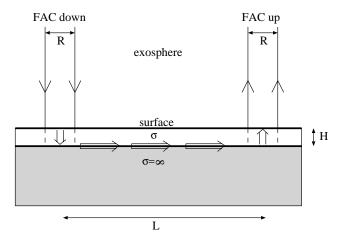
**Fig. 1.** A schematic 2-D two-layer model for FAC closure. The FAC flows into the surface on the left, moves down across a resistive surface layer (white, conductivity  $\sigma$ ) to an ideal conductor surface (gray), where it flows horizontally until it moves up on the right through the resistive layer again and emanates from the surface as an upward FAC.
