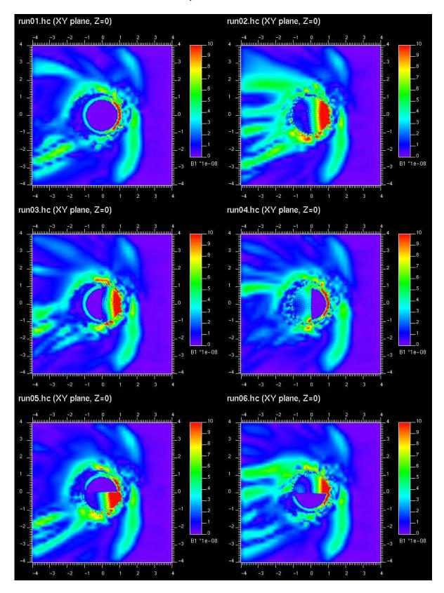
**Fig. 5.** The perturbation magnetic field  $B_1 = |\mathbf{B} - \mathbf{B}_{\text{dip}}|$  in the XY plane in all runs (for definitions of runs 1–6, see Table 1). The horizontal axis is X (Sun is to the right) and vertical is Y (growing from dawnside toward duskside). The Z axis points out of the page.
