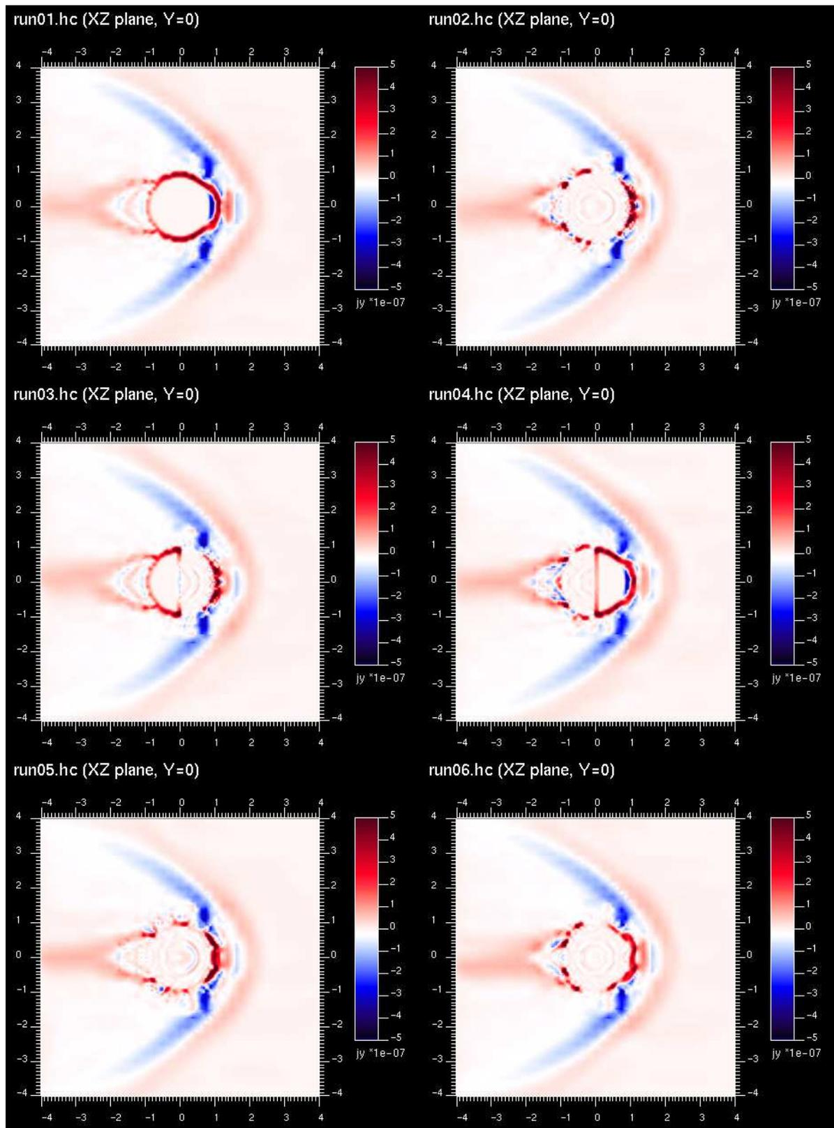
**Fig. 4.** The current density  $y$  component in the XZ plane in all runs (for definitions of runs 1–6, see Table 1). The horizontal axis is  $X$  (Sun is to the right) and vertical is  $Z$  (antiparallel to planetary dipole moment and parallel to IMF). The  $Y$  axis points toward the page.
