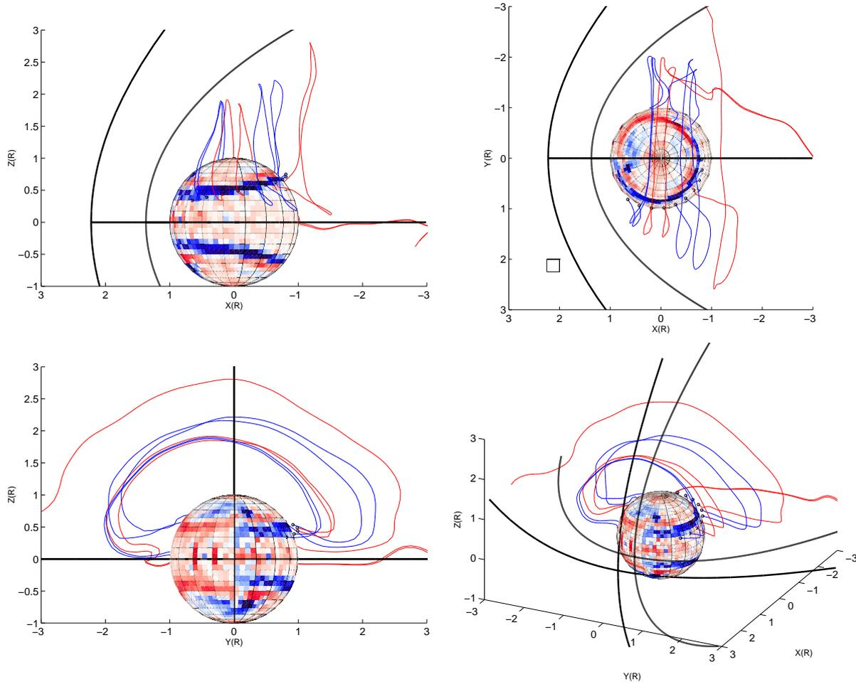
**Fig. 3.** Current lines starting from the ionosphere for run 1. The same lines are shown from four viewpoints. The starting points are selected in the duskside where significant current flows out of the planet. Lines returning to the planet are shown as blue and lines hitting the simulation box outer boundary are shown in red. To guide the eye, roughly estimated bow shock and magnetopause positions are shown as black lines.
