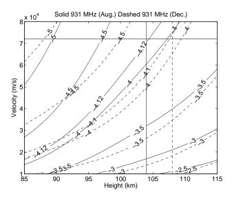
**Fig. 9.** Showing the altitude at which the ionisation produced by a meteor of a given size first reaches critical density at the EISCAT UHF frequency, 930 MHz, with log (meteor radius in meters) as a parameter. Height is related to atmospheric density through the MSISE-90 model. Solid lines represent an August atmosphere and dashed lines a December atmosphere. The vertical lines indicate the corresponding cutoff altitudes.
