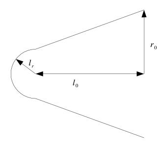
**Fig. 8.** Simplified view of the region closest to the meteor, where  $l_r$  is the mean free path length for the scattered and emitted molecules from the meteoroid,  $l_o$  is the distance the meteoroid moves before a scattered molecule becomes thermalized, and  $r_o$  is the initial trail radius. Note this drawing is not to scale.
