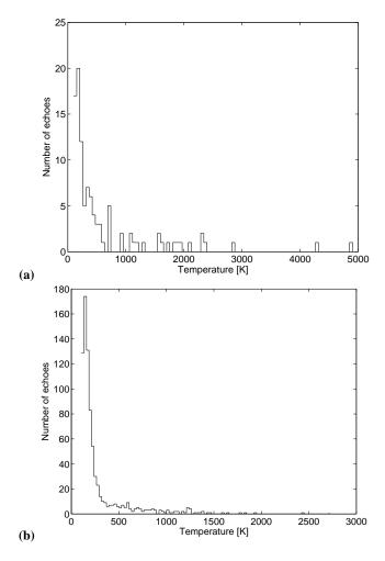
**Fig. 4.** All UHF (**a**) and VHF (**b**) head echoes as a function of the event equivalent noise temperature. The  $3\sigma$  threshold values are 30 K for the UHF and 90 K for the VHF.
