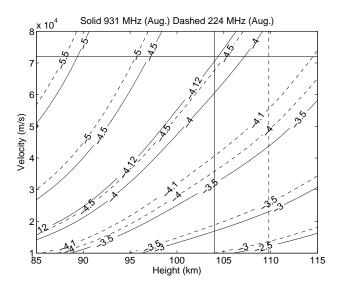
**Fig. 10.** As Fig. 9, but showing UHF and VHF (224 MHz) critical density altitudes in an August atmosphere. Dashed lines are VHF, solid lines are UHF. The vertical lines indicate the corresponding cutoff altitude.
