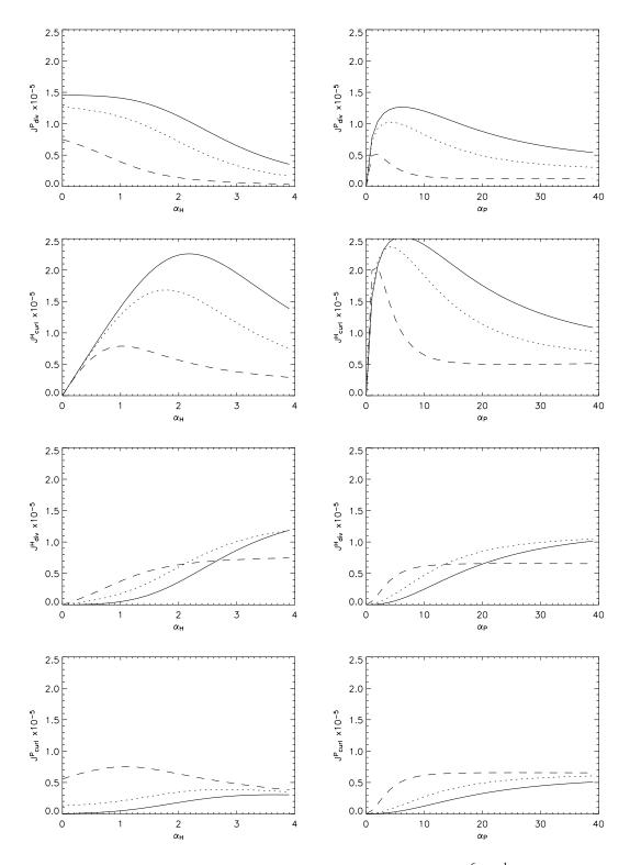
Fig. 7. The magnitude of the ionospheric current densities for the inductive effect where  $V_a = 1 \times 10^6 \text{ ms}^{-1}$ ,  $k_x = 0$ ,  $k_y = 1/d$  for d=100 km and f=40 mHz. The variation with  $\alpha_P$  has  $\alpha_H = 2$  and the variation with  $\alpha_H$  has  $\Sigma_P = 10$  S. The dip angle of **B**<sub>0</sub> is 90° (solid), 60° (dotted) and 30° (dashed) lines.
