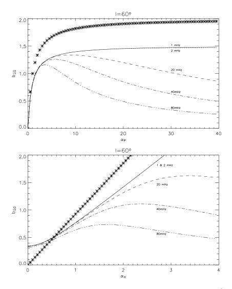
**Fig. 4.** The normalised, horizontal ULF magnetic field at the ground for a  $B_0$  dip angle of  $60^\circ$ ,  $V_a = 1 \times 10^6 \text{ ms}^{-1}$ ,  $k_x = 0$ ,  $k_y = 1/d$  and d = 100 km. (a) Variation with  $\alpha_P$  for  $\alpha_H = 2$ . (b) Variation with  $\alpha_H$  for  $\Sigma_P = 10$  S. The \* symbols show the  $\frac{\Sigma_H}{\Sigma_R + \Sigma_R}$  curve.
