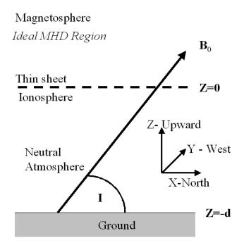
**Fig. 1.** Geometry of the magnetosphere, ionosphere and atmosphere used for the ULF wave propagation model.
