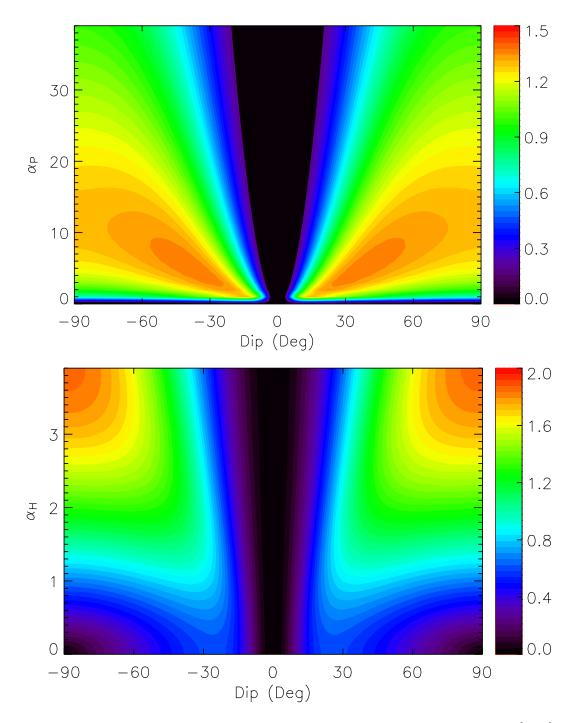
Fig. 5. The normalised, orizontal ULF magnetic field at the ground as a function of dip angle for f=20 mHz,  $V_a = 1 \times 10^6 \text{ ms}^{-1}$ ,  $k_x = 0$ ,  $k_y = 1/d$  and d=100 km. (a) Variation with  $\alpha_P$  for  $\alpha_H = 2$ . (b) Variation with  $\alpha_H$  for  $\Sigma_P = 10$  S.
