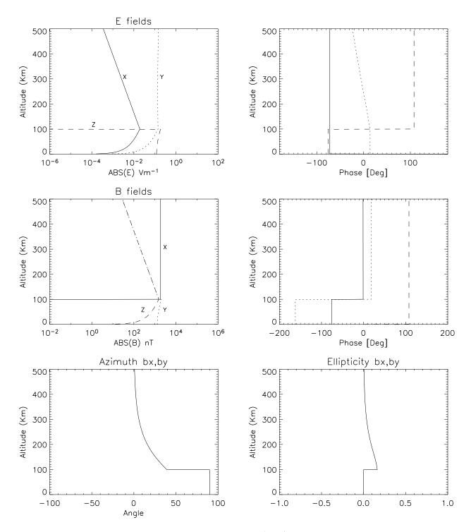
**Fig. 2.** ULF wave fields for vertical  $B_0$ ,  $k_x=0$ ,  $k_y=1/d$ , d=100 km,  $V_a=1\times10^6$  ms<sup>-1</sup>, f=20 mHz,  $\alpha_P=10$  and  $\alpha_H=20$ . The wave fields are X (solid), Y (dotted) and Z (dashed). The azimuth panel shows the NDR.
