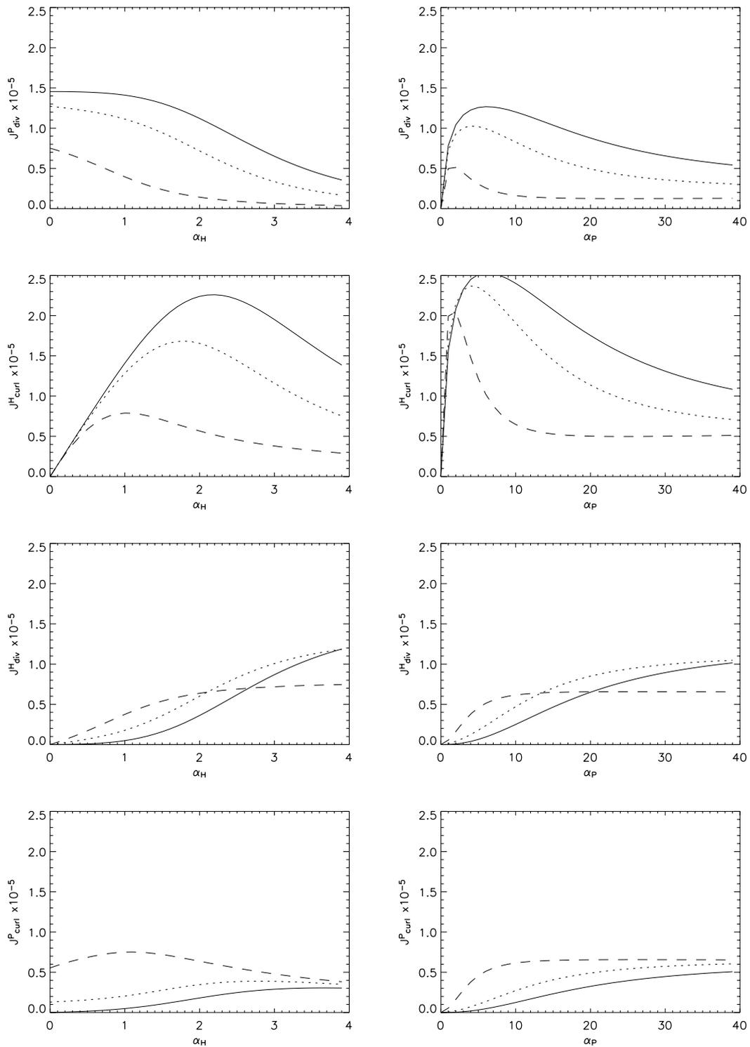
**Fig. 7.** The magnitude of the ionospheric current densities for the inductive effect where  $V_a=1 \times 10^6 \text{ ms}^{-1}$ ,  $k_x=0$ ,  $k_y=1/d$  for  $d=100 \text{ km}$  and  $f=40 \text{ mHz}$ . The variation with  $\alpha_P$  has  $\alpha_H=2$  and the variation with  $\alpha_H$  has  $\Sigma_P=10 \text{ S}$ . The dip angle of  $\mathbf{B}_0$  is  $90^\circ$  (solid),  $60^\circ$  (dotted) and  $30^\circ$  (dashed) lines.
