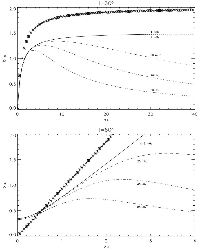
**Fig. 4.** The normalised, horizontal ULF magnetic field at the ground for a  $\mathbf{B}_0$  dip angle of  $60^\circ$ ,  $V_a=1 \times 10^6 \text{ ms}^{-1}$ ,  $k_x=0$ ,  $k_y=1/d$  and  $d=100 \text{ km}$ . **(a)** Variation with  $\alpha_P$  for  $\alpha_H=2$ . **(b)** Variation with  $\alpha_H$  for  $\Sigma_P=10 \text{ S}$ . The \* symbols show the  $\frac{\Sigma_H}{\Sigma_P+\Sigma_a}$  curve.
