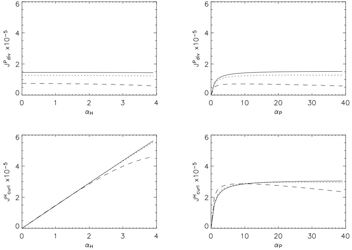
**Fig. 6.** The magnitude of the ionospheric current densities for the electrostatic approximation where  $V_a=1 \times 10^6 \text{ ms}^{-1}$ ,  $k_x=0$ ,  $k_y=1/d$  and  $d=100 \text{ km}$  and  $f=2 \text{ mHz}$ . The variation with  $\alpha_P$  has  $\alpha_H=2$  and the variation with  $\alpha_H$  has  $\Sigma_P=10 \text{ S}$ . The dip angle of  $\mathbf{B}_0$  is  $90^\circ$  (solid),  $60^\circ$  (dotted) and  $30^\circ$  (dashed) lines.
