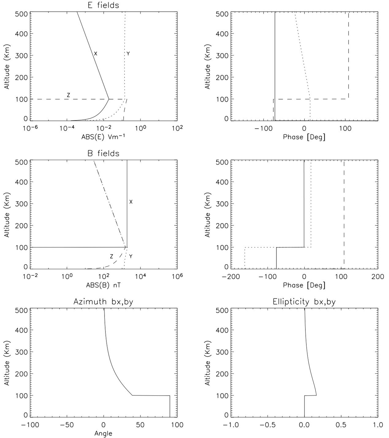
**Fig. 2.** ULF wave fields for vertical  $\mathbf{B}_0$ ,  $k_x=0$ ,  $k_y=1/d$ ,  $d=100$  km,  $V_a=1 \times 10^6$  ms $^{-1}$ ,  $f=20$  mHz,  $\alpha_P=10$  and  $\alpha_H=20$ . The wave fields are X (solid), Y (dotted) and Z (dashed). The azimuth panel shows the NDR.
