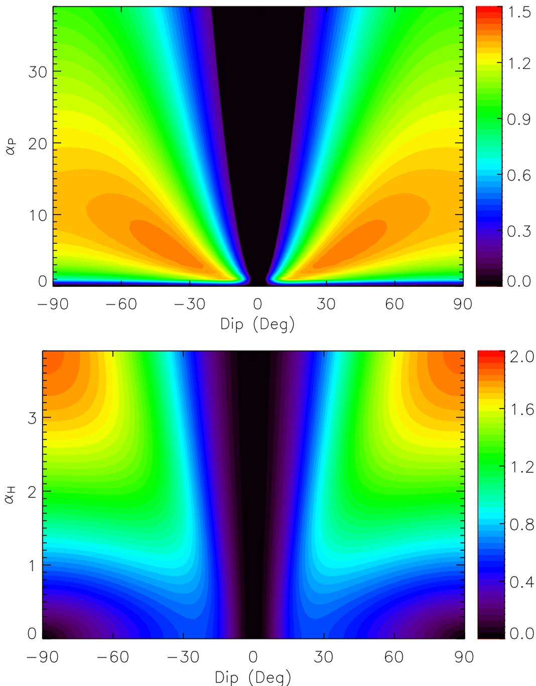
**Fig. 5.** The normalised, horizontal ULF magnetic field at the ground as a function of dip angle for  $f=20$  mHz,  $V_a=1\times 10^6$  ms $^{-1}$ ,  $k_x=0$ ,  $k_y=1/d$  and  $d=100$  km. **(a)** Variation with  $\alpha_P$  for  $\alpha_H=2$ . **(b)** Variation with  $\alpha_H$  for  $\Sigma_P=10$  S.
