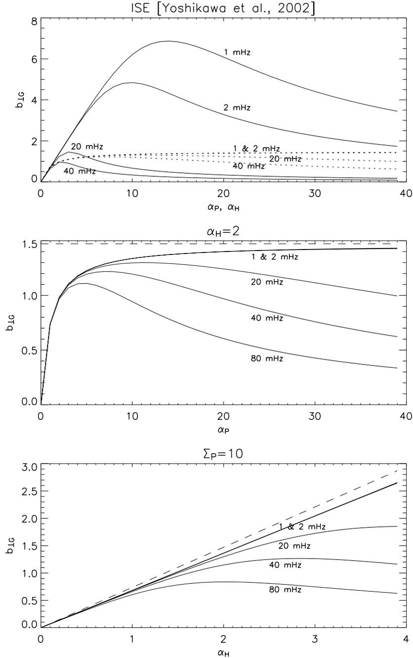
**Fig. 3.** The normalised, horizontal ULF magnetic field at the ground for vertical  $\mathbf{B}_0$ ,  $V_a=1 \times 10^6 \text{ ms}^{-1}$ ,  $k_x=0$ ,  $k_y=1/d$  and  $d=100 \text{ km}$ . (a) variation with  $\alpha_P$  (dotted) and  $\alpha_H$  (solid) for the parameters in Yoshikawa et al. (2002). (b) Variation with  $\alpha_P$  for  $\alpha_H=2$ . (c) Variation with  $\alpha_H$  for  $\Sigma_P=10 \text{ S}$ .
