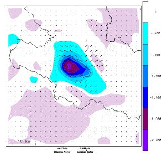
**Fig. 4.** Near surface temperature (color shading) and wind (arrows) difference between the SUMWF lake and corresponding no-lake cases at 02 July 1999, 12:00 GMT. Units are K for temperature and m/s for wind speed.
