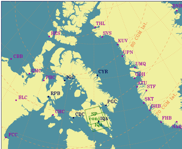
Fig. 6. Map of arctic Canada and western Greenland. Locations of magnetometer stations are indicated with filled circles, those in dark blue provided data shown in this paper, those in violet are included for completeness. Imaging riometers are indicated with outlined squares which represent their approximate field-of-view. The conjugate position of the South Pole (SP conj) was calculated with T96, see Sect. 3.1. Dotted lines comprise a geographic grid with 5° divisions in latitude and 10° in longitude. CGM latitude contours in dashed lines are also plotted.
