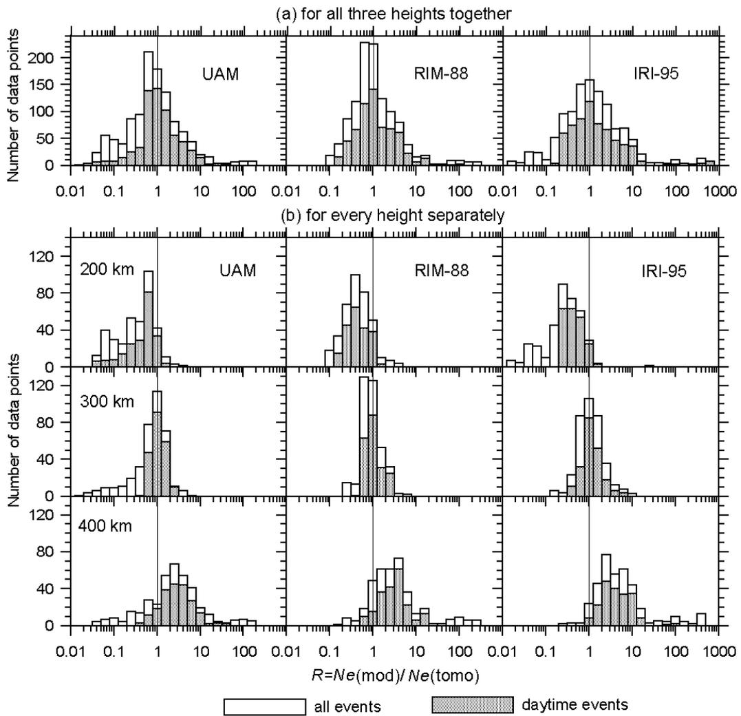
**Fig. 11.** Histograms of the ratios of the model electron density to the electron density measured by the radio tomography,  $R = N_e(\text{mod})/N_e(\text{tomo})$ , for three ionosphere models: the theoretical model UAM (left column) and two empirical models RIM-88 (middle column) and IRI-95 (right column). **(a)** For all three heights together (200, 300 and 400 km). **(b)** For every height separately.
