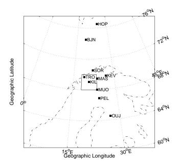
**Fig. 1.** The locations of the instruments used in this study. IMAGE magnetometers are indicated by the squares. The box centred on station KIL represents the IRIS field-of-view as used for the images in this paper.
