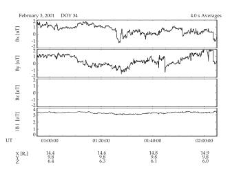
**Fig. 8.** Magnetic field measurements made on board the Cluster 1 spacecraft in the time interval 3 February 2001, 00:55–02:03 UT.
