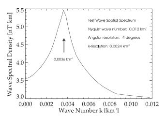
**Fig. 2.** Shell-max spatial spectral density distribution in logarithmic presentation resulting from applying the wave telescope to the artificial data set.
