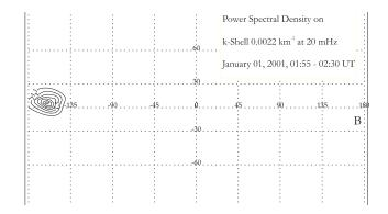
**Fig. 6.** Spectral density distribution on the k-shell  $k = 0.0022 \,\mathrm{km}^{-1}$  resulting from applying the wave telescope to measurements in the magnetosheath during the interval 1 January 2001, 01:55–02:30 UT. The logarithm of the power is displayed. 'B' denotes the position of the mean magnetic field direction.
