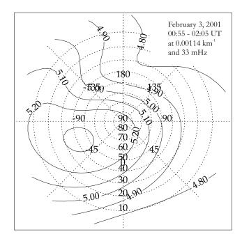
**Fig. 11.** Spectral density distribution on the k-shell  $k = 0.00115 \, \mathrm{km}^{-1}$  resulting from applying the wave telescope to measurements in the solar wind during the interval on 3 February 2001, 00:55–02:05 UT. The logarithm of the power, given in pT, is displayed.
