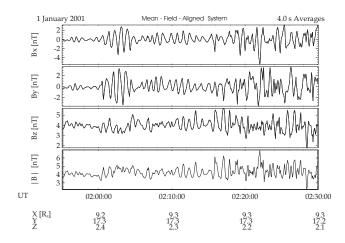
**Fig. 4.** Magnetic field observations recorded by Cluster 1 in the interval on 1 January 2001, 01:55–02:30 UT. The data are displayed in a mean field-aligned coordinate system with the  $B_Z$  direction aligned with the mean magnetic field direction.
