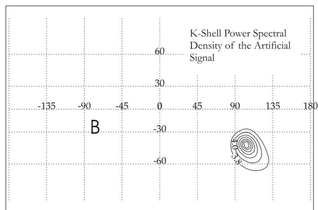
**Fig. 3.** Distribution of power on the  $k$ -shell  $k = 0.0036 \text{ km}^{-1}$  in a stereographic projection and logarithmic representation.  $B$  denotes the position of the mean magnetic field direction.
