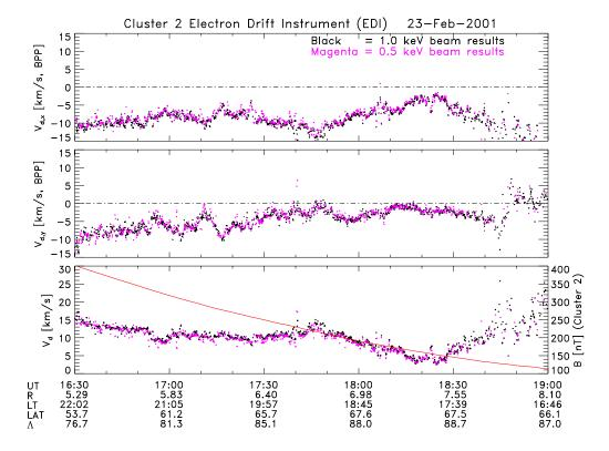
Fig. 11. Comparison of the drift velocities measured at 0.5 and 1.0 keV for the pass on 23 February, 16:30–19:00 UT. The plot shows the two components of the drift in the  $B_{\perp}$ -plane, plus the magnitude. The magnitude of B is shown superimposed in the bottom panel.
