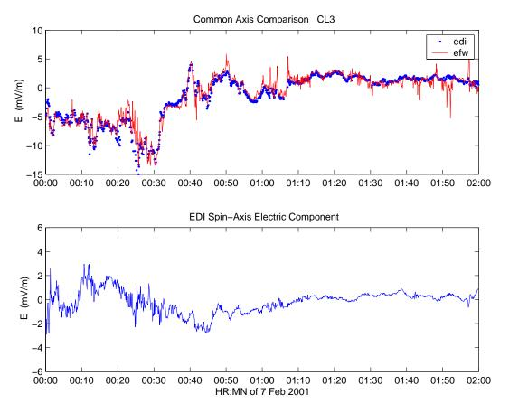
**Fig. 15.** Comparison of EDI and EFW electric fields. The top panel shows the component of *E* along the common axis defined in the text. The bottom panel shows the spin axis component measured by EDI.
