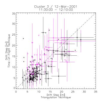
**Fig. 9.** Scatter plot of the drift speeds derived by the time-of-flight analysis (vertical axis) against those from the triangulation analysis (horizontal axis), for the interval 11:30 through 12:10 on 12 March 2001, on SC 3. The two types of symbols refer to the different time-of-flight analysis methods, as in Fig. 8. Error bars are only shown for a fraction of the points so as not to clutter the figure.
