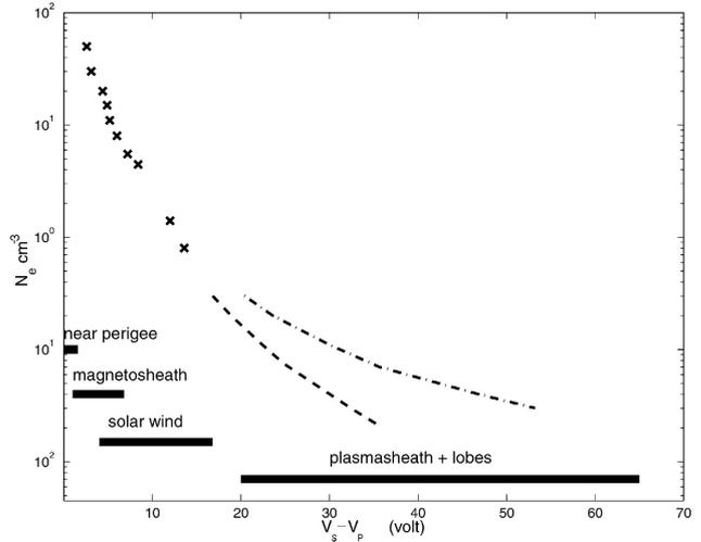
**Fig. 2.** Calibration of the spacecraft to-probe-potential difference ( $V_S - V_P$ ) in solar wind with electron densities measured by Whisper (crosses). Dotted lines indicate the expected range of ( $V_S - V_P$ ) in the plasmasheath and lobes, to be calibrated later with particle experiments.
