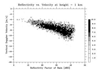
**Fig. 3.** Frequency distribution of the equivalent radar reflectivity vs. vertical Doppler velocity at 1 km height for all BLR data when the surface raingauge detected rain from November 1992 to December 1998.
