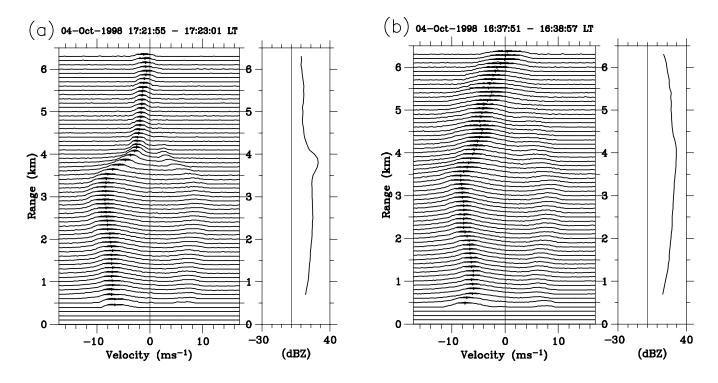
**Fig. 2.** Doppler spectra obtained by a vertical beam of Bukittinggi BLR at (a) 1721 LT and (b) 1637 LT on 4 October 1998. Left panels are the Doppler velocity spectra with thick vertical lines, indicating mean Doppler velocity and thick horizontal lines representing spectral width. The vertical profiles of equivalent radar reflectivity are plotted in the right panels.
