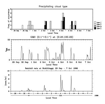
Fig. 5. (a) Occurrence frequency of precipitating clouds classified from BLR data every 3 hours. (b)  $T_{\rm BB}$  index from GMS-IR at (0.2° S, 100.3° E). (c) Rainfall rate averaged every 1 hour.
