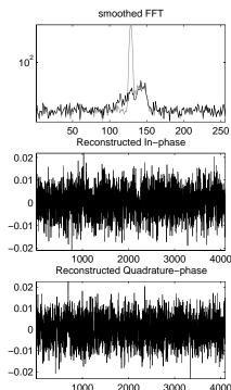
Fig. 8. Top left: Simulated Fourier-power-spectrum with strong ground clutter influence and with an atmospheric signal overlapping the ground clutter peak. Lower left: I/Q time series derived from the simulated Fourier-power-spectrum using the Zrnić (1975) method. Lower right: I/Q time series after applying the nonlinear wavelet filter. Top right: Resulting Fourier-power-spectrum based on the reconstructed (filtered) signal.
