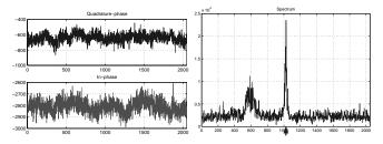
**Fig. 3.** The left part shows the "stacked spectrum" plot, i.e. the Doppler spectra for each range gate, for the radar dwell at 08:53:38 UTC on 1 December 1999. The right figures give a detailed look into the raw data (I/Q-timeseries) and the Doppler spectrum for the gates 11 and 17 (whose data will be wavelet processed). The black arrows indicate the estimated first moment (i.e. the radial velocity).
