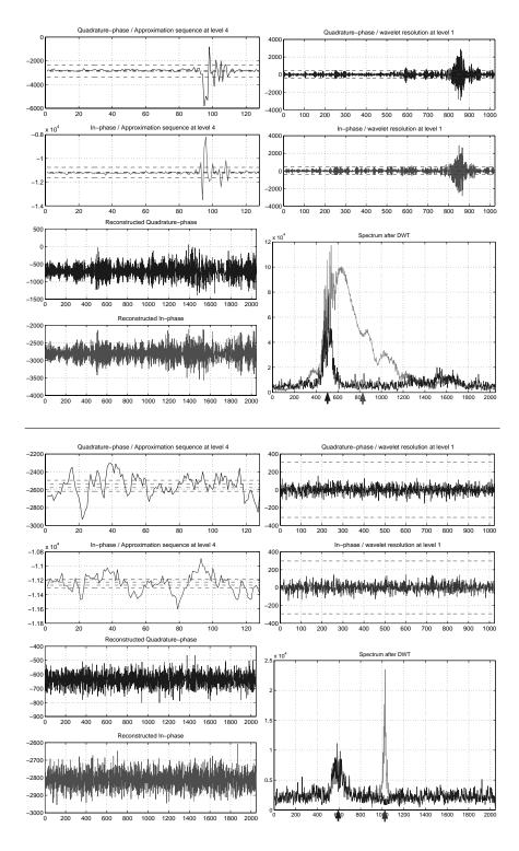
Fig. 7. Decomposition ( $\alpha_k$  und  $\beta_{1k}$ ), reconstruction and Fourier power spectrum of gate 17 (top) and gate 11 (below). The black curves in the power spectra representations display the decontaminated spectra. One clearly recognizes are the differences of moment estimations; see the computed first moment before (gray arrow) and after (black arrow) the filtering step.
