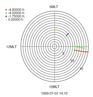
**Fig. 6.** Back-tracing of the ion cloud at 3 July, 14:15 UT. The exterior of the cloud is specified by energy, MLT and L-shell. The drift-velocities are given by Eq. (1). Yellow color corresponds to the measured event, while red color corresponds to the estimated time of injection (4.8 hours before).
