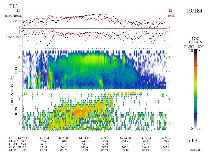
Fig. 8. DMSP F13 particle data from the conjugate point of the ion cloud observed by Astrid-2 on 3 July 1999, 14:15 (see Fig. 1). Color scale is differential energy flux in  $eV/(cm^2 \text{ s ster } eV)$ . (Courtesy Pat Newell)
