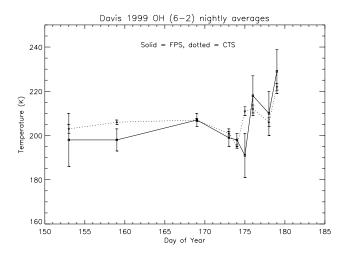
**Fig. 4.** Mean nightly temperatures from the OH(6–2) observations using the CTS (dotted line) and FPS (solid line), Davis, June 1999. One-sigma standard errors are shown. The absolute values of the FPS temperatures have been adjusted to make the nightly mean for DOY 169 equal to the CTS mean for that night. See the text.
