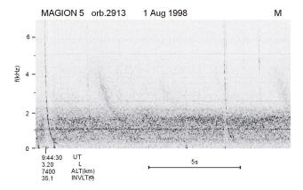
**Fig. 6.** VLF wave spectrograms from a short interval of the MA-GION 5 orbit No. 2913 (see Fig. 5, upper panel). Electric and magnetic components are shown in the upper and lower panels, respectively. LHR noise band is observed in the E- component only.
