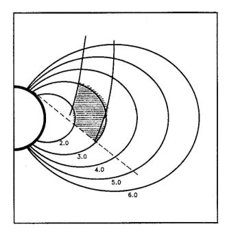
**Fig. 4.** Parts of MAGION 4 orbits, the lowest and the highest ones, on which magnetospherically reflected whistlers were observed. Dashed line is the limit of real time telemetry zone of the Panská Ves station where the analog broadband signal 0.1–22 kHz was recorded. The region of MR whistler occurrence is denoted by hatching.
