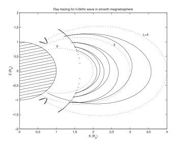
**Fig. 8.** Propagation paths for the wave with frequency  $f=5\,\mathrm{kHz}$  calculated without taking into account the plasmapause. The contour corresponding to LHR frequency 5 kHz in the model used in calculations is shown by dotted line.
