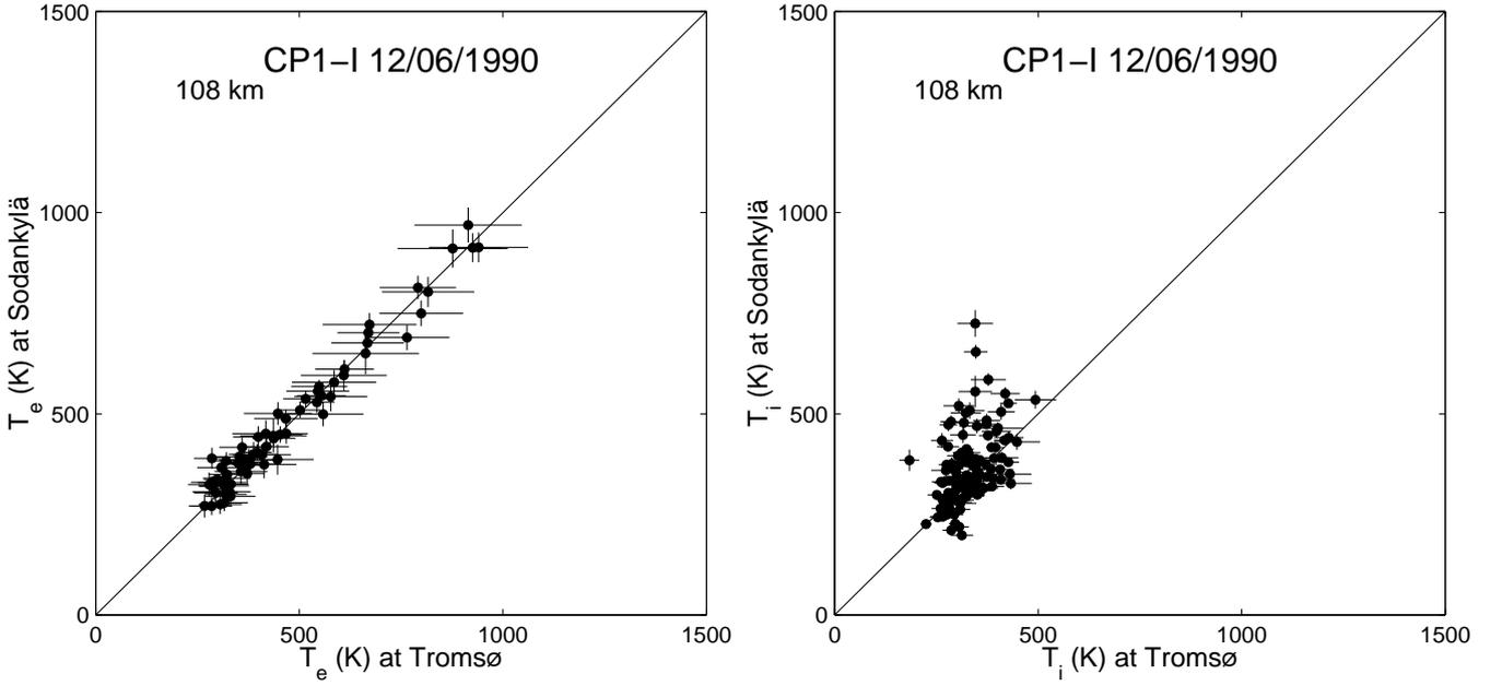
**Fig. 2.** Left panel: Scatter plot of the electron temperatures from different aspect angles observed with the Tromsø and Sodankylä EISCAT sites. The errors in fitting to the IS spectra are also plotted. Right panel: The same as the left panel, but the ion temperatures are compared.
