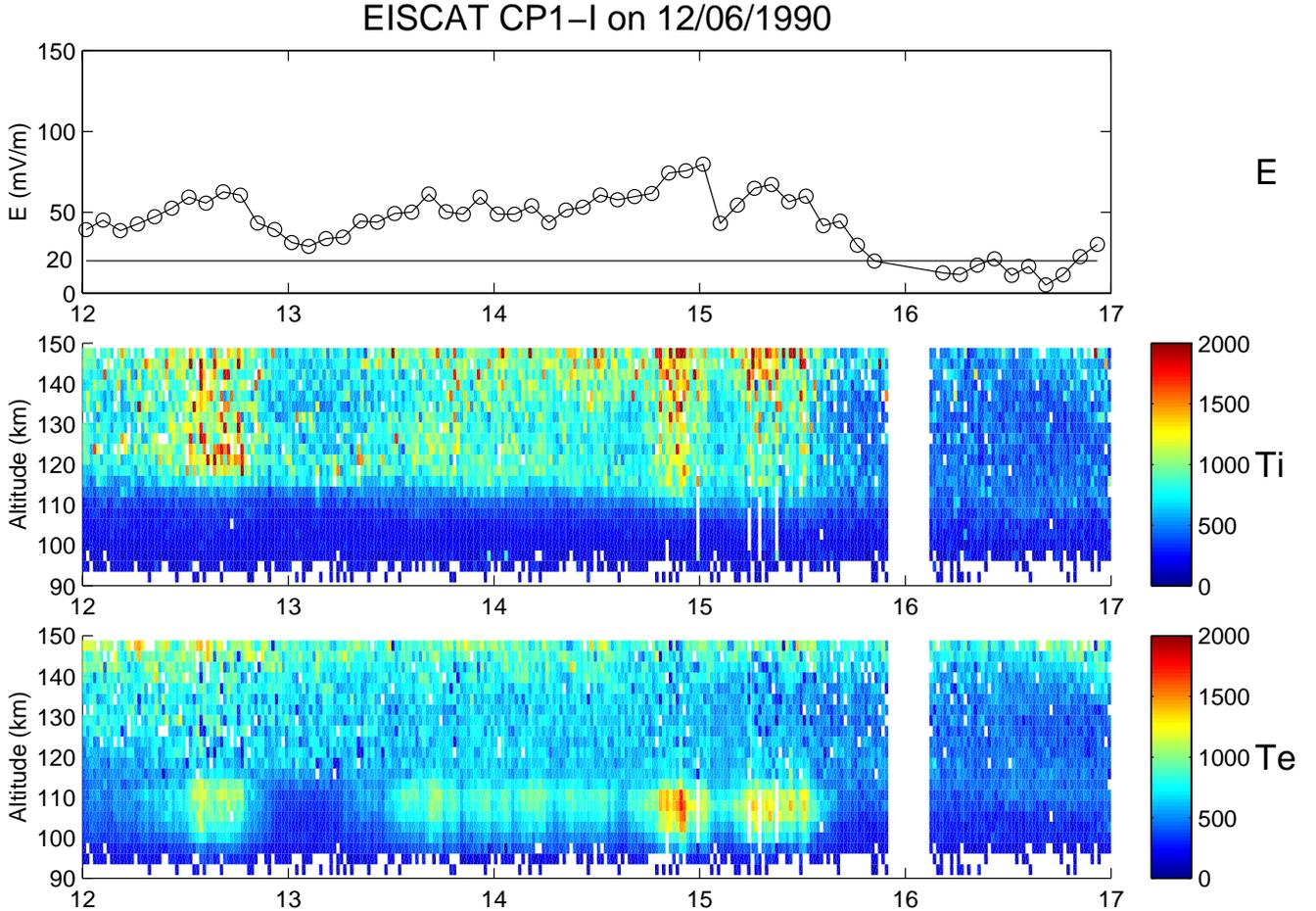
**Fig. 1.** Overview of a data set with long periods of elevated  $T_e$  in the lower E region. The top panel shows  $|E|$  with a time resolution of 5 minutes. The approximate threshold of the MTSI is about  $20 \text{ mV m}^{-1}$ . The middle and bottom panels show the electron and ion temperatures, respectively.
