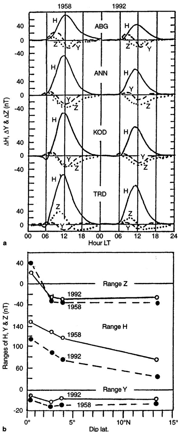
Fig. 1. Annual mean solar daily variations of the three components of the geomagnetic field, horizontal ( $H$ ), eastward ( $Y$ ) and vertical ( $Z$ ) for the years 1958 and 1992 at the four observatories in India. Trivandrum (TRD), Kodaikanal (KOD), Annamalainagar (ANN), and Alibag (ABG)
