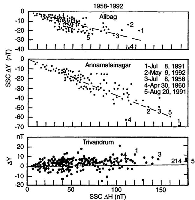
Fig. 7. Relationship between amplitudes of SSC  $\Delta Y$  and  $\Delta H$  at the stations Annamalainagar (*ANN*) Trivandrum (*TRD*) and Alibag (*ABG*) of SSCs for 1958–1992
