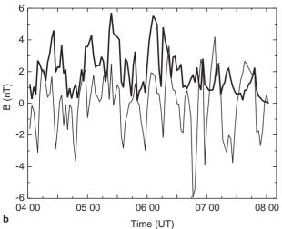
Fig. 6a, b. Magnetic field variations along and transversely to the background magnetic field for the same intervals as for Fig. 5. The solid lines correspond to compressional component and dashed lines correspond to transverse component
