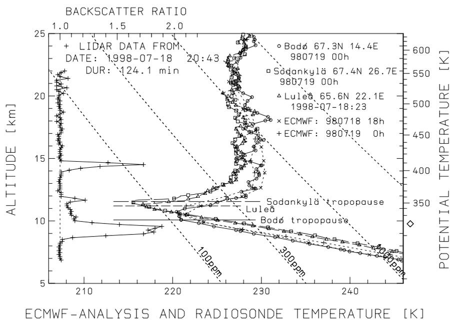
**Fig. 1.** The left points show the lidar backscatter ratio at wavelength 532 nm averaged in time from 2043 to 2247 UT on July 18, 1998. Temperature profiles (right curves) from ECMWF analyses and the midnight radiosondes launched at Bodø, 290 km west of Esrange, Sodankylä, 245 km east, and Luleå, 265 km south. Dashed oblique lines give water vapour saturation temperatures for hypothetical assumptions about stratospheric water vapour mixing ratios from 100 to 3000 ppmv
