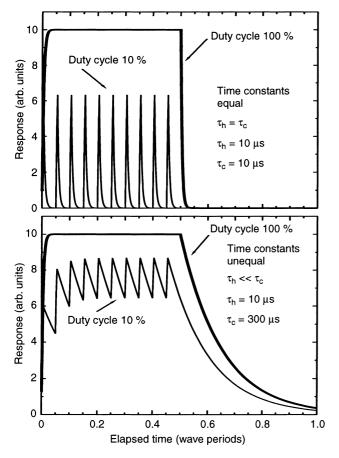
**Fig. 4.** ELF pulse response of ionosphere to heating with waveforms of 10 and 100% duty cycle. *Upper panel*: heating and cooling time constants of ionospheric current both =  $10 \,\mu$ s. *Lower panel*: heating time constant =  $10 \,\mu$ s. Cooling time constant =  $300 \,\mu$ s
