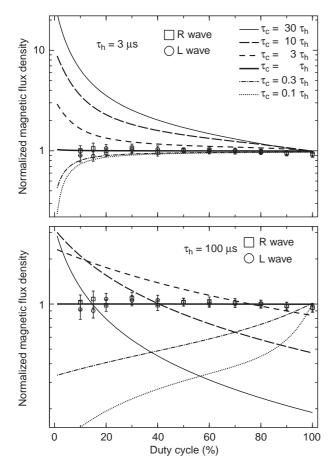
**Fig. 6.** Theoretical estimates of normalised magnetic flux density at 505 Hz produced by modulated ionospheric currents, plotted for a range of six cooling time constants. *Upper panel* data computed for a heating time constant of  $3 \mu s$ . *Lower panel* data computed for a heating time constant of 100  $\mu s$ . The *square* and *round markers*, with their associated *error bars*, represent the experimentally measured 'R' and 'L' wave normalised magnetic flux densities respectively
