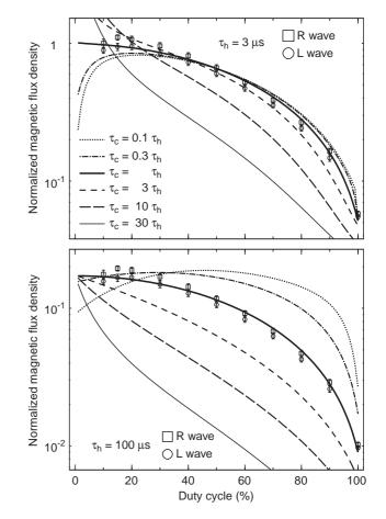
Fig. 7. Theoretical estimates of normalised magnetic flux density at 9595 Hz produced by modulated ionospheric currents, plotted for a range of six cooling time constants. *Upper panel* data computed for a heating time constant of  $3 \mu s$ . *Lower panel* data computed for a heating time constant of 100  $\mu s$ . The *square* and *round markers*, with their associated *error bars*, represent the experimentally measured 'R' and 'L' wave normalised magnetic flux densities respectively
