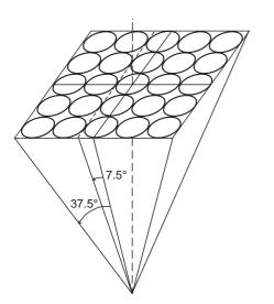
Fig. 1. Technique for enhancing ELF radiated power by scanning the HF beam over an area within the antenna beam angle of  $\pm 37.5^{\circ}$  (see Papadopoulos *et al.*, 1989)
