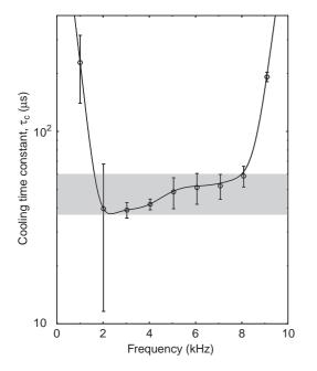
Fig. 14. Cooling time constants derived from first nine even harmonics of 505 Hz. Grey shaded area shows range in which more than 75% of data points are accommodated
