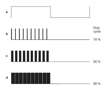
**Fig. 3.** HF heater transmitter keying waveform. **a** desired ELF current in ionosphere, **b**-**d** effective HF output from heater transmitter with pulsed amplitude modulation of 10, 50 and 90% duty cycle respectively
