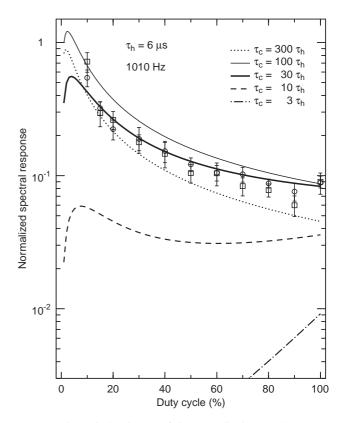
Fig. 12. Theoretical estimates of the normalised spectral response at 1010 Hz plotted for a heating time constant of  $6 \,\mu s$  and a range of five cooling time constants. The square and round markers, with their associated error bars, represent the experimentally measured 'R' and 'L' wave normalised spectral responses respectively
