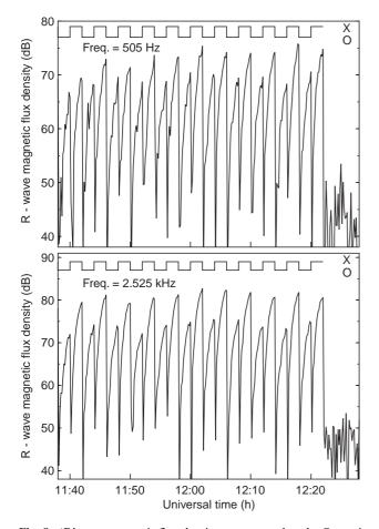
**Fig. 8.** 'R' wave magnetic flux density as measured at the Oststation. *Upper panel*: Measurements at the fundamental frequency of 505 Hz. *Lower panel*: Measurements at the harmonic frequency of 2525 Hz. The crenellated waveform at the top of each panel shows when the heater transmitter was switched between 'X' and 'O' mode transmissions
