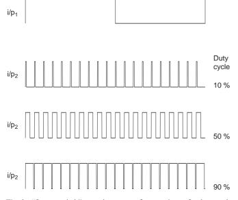
**Fig. 2.** "Sousy switch" gate input waveforms.  $i/p_1$  – fundamental ELF waveform, typically 505 Hz.  $i/p_2$  – variable duty cycle waveform (0–100%), typically 10.1 kHz
