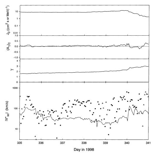
Fig. 4. Detail of the zero anisotropy phase and calculation of the speed of the frame of scattering centres. For channel 7 are shown the omnidirectional flux  $J_0$ ,  $(A_I)_{\parallel}$ , the spectral index  $\gamma$  and the speed of scattering centres  $|V_{sc}^*|$ . In the lowest plot solid circles indicate anti-Sunward motion of the scattering centres and open triangles Sunward motion
