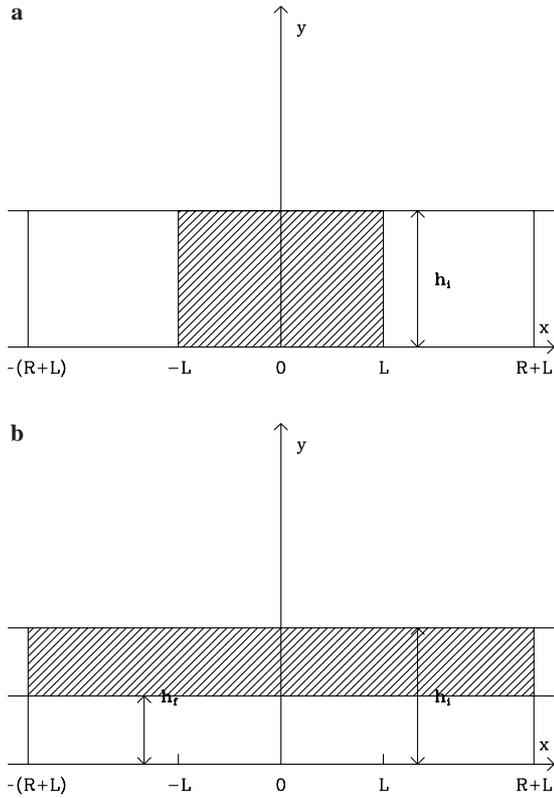
**Fig. 3.** **a** Air masses in a heated boundary layer over a flat peninsula.  $h_i$  is the initial boundary layer depth,  $2L$  is the patch width and  $R$  is the Rossby radius. **b** As in **a** but after the adiabatic redistribution of air masses.  $h_f$  is defined by mass conservation.  $R$  and  $L$  as in **a**
