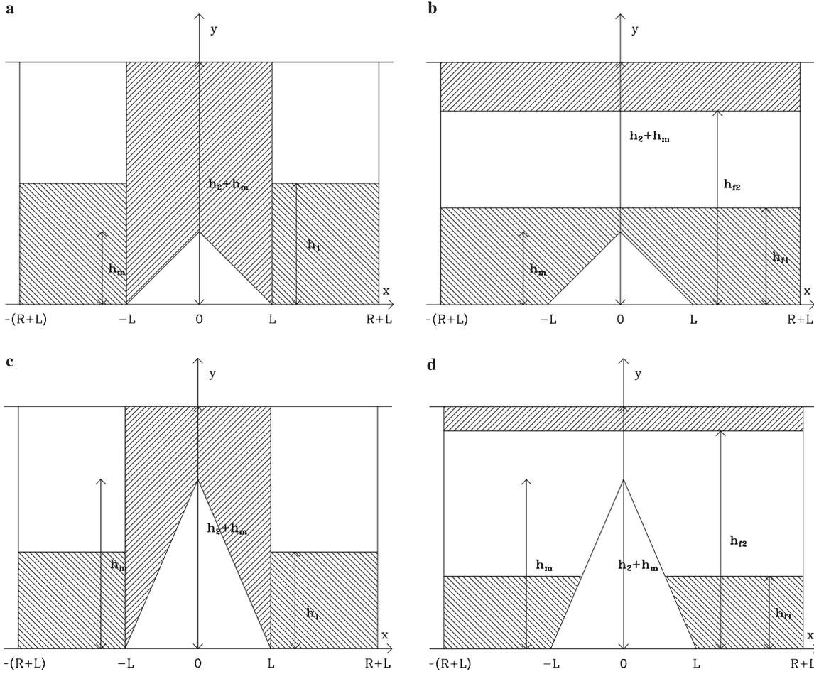
**Fig. 5.** **a** Air masses in two heated boundary layer over mountainous terrain, for a small mountain.  $h_m$  is the mountain height.  $R$  and  $L$  as in Fig. 3a.  $h_2$  is the boundary layer depth over the mountain and  $h_1$  is the boundary layer depth over the flat terrain. **b** As in **a** but after an
