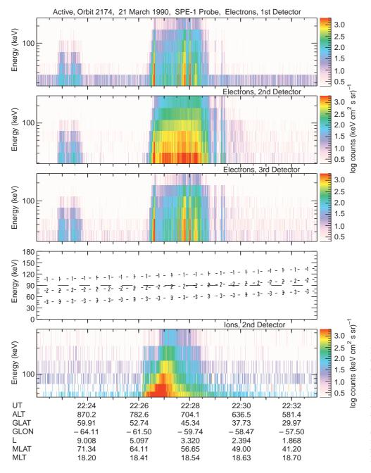
Fig. 7. SPE-1 energetic electron (*upper three panels*) and ion (*bottom*) spectra measured with three different detectors whose pitch angle orientations are given in the *fourth panel*. At the abscissa are shown the satellite's altitude (*ALT*), geographic latitude (*GLAT*) and longitude (*GLON*), the *L*-value, geomagnetic latitude (*MLAT*) and the magnetic local time in decimal hours (*MLT*)
