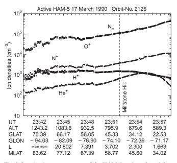
**Fig. 2.** Ion density measurements of the HAM-5 probe onboard the Active satellite along the orbit 2125 path. This passed the Millstone Hill station within a horizontal distance of the path projection to the Earth's surface of 160 km just prior to the first storm onset during local sunset (23:52 UT) on 17 March 1990. See Fig. 3 for the direct comparison with the radar measurements
