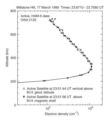
Fig. 3. Direct comparison of electron density measurements of the HAM-5 probe onboard the Active satellite with the measured Millstone Hill  $N_e$  radar profile for the direct overflight during orbit 2125 on March 17, 1990, a geomagnetically quiet prestorm day
