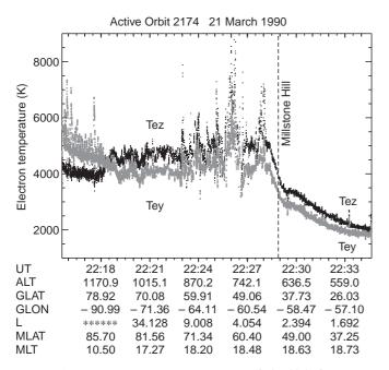
**Fig. 6.** Electron temperature measurements of the high frequency probe KM-6 along orbit 2174 of the Active main satellite on March 21, 1990 during its passage near the Millstone Hill station.  $T_{ex}$  is the temperature component measured vertically upward;  $T_{ey}$  is measured horizontally and perpendicular to the flight direction
