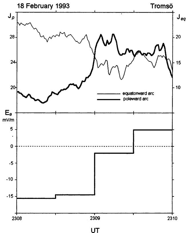
Fig. 8. Variations of the mean value of the luminosity in the system of two parallel auroral arcs (top panel) and variation of the azimuthal component of electric field in the ionosphere (bottom panel). J means the intensity of the luminosity (arbitrary units)
