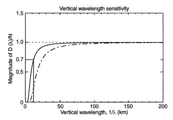
**Fig. 1.** The sensitivity of the South Pole meteor radar system to waves with differing vertical wavelengths is shown. The *solid line* (*dashed line*) indicates the sensitivity assuming a meteor region with a halfwidth of 10 km (20 km). The *solid vertical line* indicates the 3 dB point for the 10 km meteor region which occurs at a vertical wavelength of 12 km
