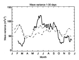
**Fig. 4.** The total variance (m<sup>2</sup> s<sup>-2</sup>) is shown computed from the South Pole observations during 1995 (*solid*) for waves with periods between 1 and 30 days. The variance is computed for every other day throughout the year utilizing 30 days of daily averaged data. Also shown are the meridional (*dashed*) and zonal (*dash-dot*) estimated wave variances computed using meteor data from Molodezhnaya (68°S) for 1986 through 1991
