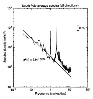
**Fig. 7.** The estimated South Pole power spectra for periods between 1 h and 30 days averaged over all four azimuth directions. The *solid line* is an estimate of the spectral trend between 1 and 30 days assuming a  $f^{-k}$  type of dependence
