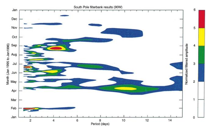
Fig. 9. The result of filtering the South Pole observations from the  $90^{\circ}$  west direction using a constant-Q filter bank. The *color key* is used to indicate statistical significance in terms of  $\sigma$
