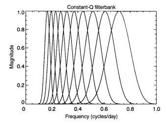
Fig. 5. An example of a constant-Q filterbank
