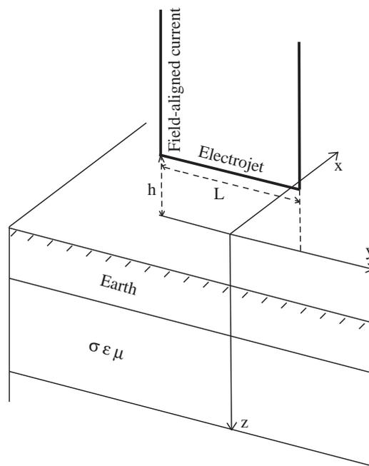
**Fig. 1.** Electrojet (amplitude  $I$ ) of a finite length  $L$  supplemented by vertical currents at the ends. The height of the electrojet is  $h$ , and the standard coordinate system with the earth’s surface as the  $xy$ -plane, the  $z$ -axis downward and the  $y$ -axis parallel to the electrojet is used in this paper
