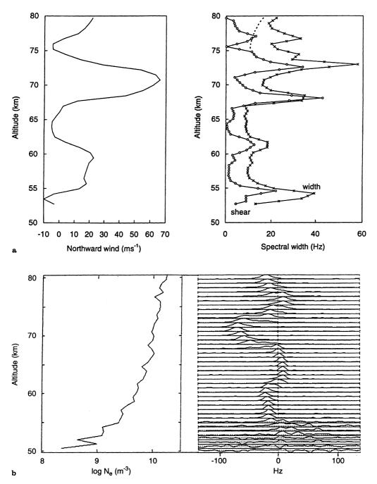
**Fig. 5. a** As Fig. 3, but for an antenna elevation of  $45^{\circ}$  at 1330 UT. **b.** The *right panel* shows measured VHF power spectra (arbitrary linear power scale) for the same time as part a. Each spectrum is
