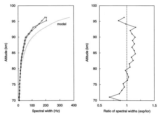
**Fig. 2.** The *left panel* shows measurements of spectral width by the EISCAT VHF radar with a vertically pointing antenna compared with model values. The profile *with open square symbols* ( $\Box$ ) is from the results of fitting exponential curves to the ACFs while that with *crosses* (x) shows the results of fitting Lorentzian curves to the spectra.
