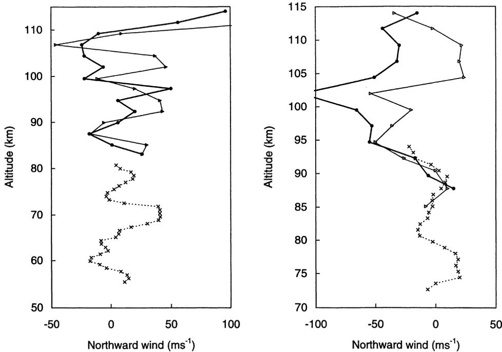
**Fig. 8.** Two examples of horizontal meridional wind measured simultaneously by the UHF and VHF radars on 20 March 1990. The VHF profiles are from a 2-min integration while the UHF results are averages over 70-s dwells in four successive 6-min scans (individual UHF profiles tend to be noisy due to the lower snr). The meridional wind derived from the S position (●) will be more
