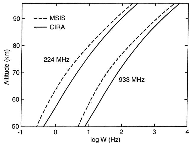
**Fig. 1.** Calculated incoherent-scatter spectral widths ( $W$ ) in the upper mesosphere for the EISCAT UHF (933 MHz) and VHF (224 MHz) radars, for the CIRA-72 (full lines) and extrapolated MSIS-83 (broken lines) atmospheric models, assuming no negative ions present
