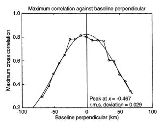
**Fig. 4.** The maximum correlation coefficient for different values of the perpendicular baseline. Each point represents the analysis of 5 min observation. The Gaussian curve fitted to these points has a peak value for  $b_{\perp} \sim 0.5$  km (as in Fig. 2) but in this case the standard error in each point  $\sigma_5 = 0.029$  (the ratio  $\sigma_5:\sigma_{10}$  is very close to  $\sqrt{2}$  so there is no evidence that the errors are other than random)
