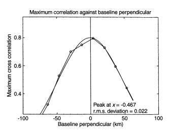
**Fig. 2.** The maximum correlation coefficient for different values of  $b_{\perp}$ , the perpendicular baseline. Each point represents the analysis of 10 min observation. The Gaussian curve fitted to these points has a peak value for  $b_{\perp} \sim 0.5$  km and the standard error in each point  $\sigma_{10} = 0.022$  (after allowing for the loss of 3 degrees of freedom in fitting)
