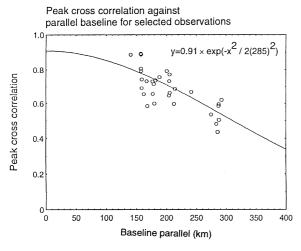
**Fig. 3.** The fall in maximum correlation coefficient as the parallel baseline increases. In this figure only high-latitude observations in which the fast-stream was >85% dominant are shown. A Gaussian curve is fitted which gave the best least-squares fit out of a straight line, and exponential decay curve and a Gaussian curve
