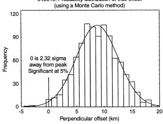
**Fig. 5.** Two examples where a Gaussian curve is fitted to the histogram of uncertainty generated by the Monte Carlo method. In the first case the parallel baseline was constant throughout the observations so there was no baseline correction. In the second case the uncertainty was greater due to the uncertainty in baseline correction. The offset is significant as 1% and 5% respectively.
