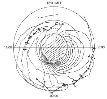
**Fig. 6.** Dial plot showing the average position of the postmidnight mid-latitude trough and the dayside trough during the quiet geomagnetic conditions as a function of corrected geomagnetic latitude (60–90°CGM) and MLT. The *squares* indicate the location of the trough minimum and the *arrows* the associated standard deviation. Superimposed is the IZMEM electric potential contours at 5-kV intervals for the mean IMF of the quiet period
