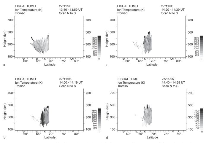
Fig. 10a-d. Ion temperatures measured by the EISCAT radar observing in the TOMO special programme mode for a series of scans between 13:40 and 15:00 UT on 27 November 1995
