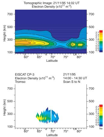
Corresponding electron densities measured by the EISCAT radar observing in the CP3 common programme mode for scans from 12:30 to 13:00 UT and 14:00 to 14:30 UT (*lower panels*)
