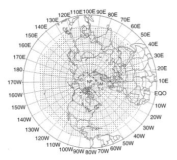
**Fig. 1.** NMC grid used in the Adem thermodynamic model: 1977 points distributed in a polar stereographic projection where *X* and *Y* coordinate axes were arbitrarily determinated along  $10^{\circ}$ E and  $80^{\circ}$ W, respectively
