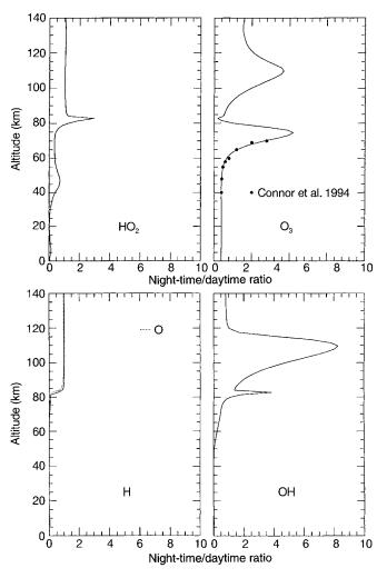
Fig. 8. Model night-time/daytime ratios for the  $HO_x$  species and for  $O_3$ . Solid circles are the ground-based microwave  $O_3$  ratio observations of Connor et al. (1994)
