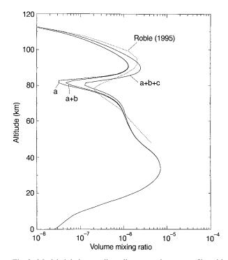
**Fig. 3.** Model global mean diurnally averaged ozone profiles with and without channels a, b and c of the reaction  $H + HO_2$ , using a Lymanalpha water-vapour photodissociation branching ratio  $\alpha = 1$
