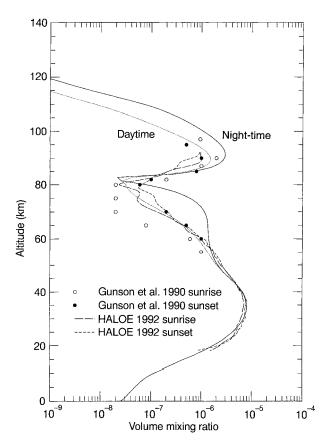
**Fig. 7.** Global mean daytime and night-time averaged ozone profiles computed by the model are compared with the sunrise and sunset measurements obtained by the ATMOS experiment on Spacelab 3 as given in Gunson *et al.* (1990) and by UARS/HALOE
