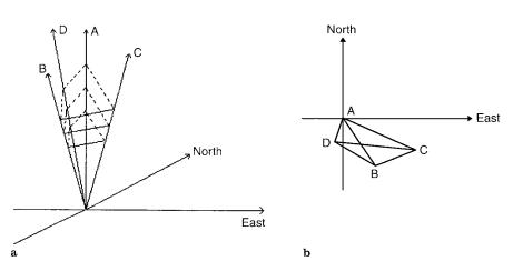
Fig. 1a, b. Illustration of the EISCAT CP2 mode: a the four probing directions of the antenna beam during CP2; b geometric configuration of the four probing positions in a plane at a fixed altitude
