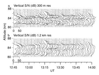
**Fig. 4a, b.** Altitude profiles of the vertical S/N at a 300-m-altitude resolution and b 1.2-km-altitude resolution on 22 June 1994
