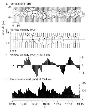
**Fig. 1a–d.** Altitude profiles of **a** the vertical S/N and **b** vertical velocity on 17 June 1993. The *bold profiles* correspond to the times at which the sense of the vertical velocity reverses. Also shown are the variations in **c** of the vertical velocity and **d** horizontal speed at an altitude of 85.4 km, indicated by the *horizontal lines* in a and b
