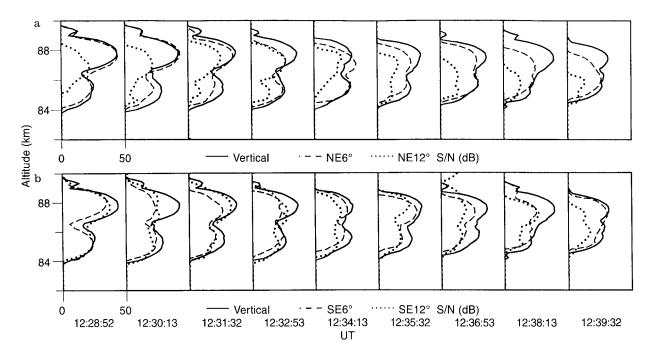
Fig. 8a, b. Altitude profiles of the S/N for the vertical and  $6^{\circ}$  and  $12^{\circ}$  beams in a the NE azimuth and b SE azimuth for nine consecutive cycles of observation on 8 July 1993
