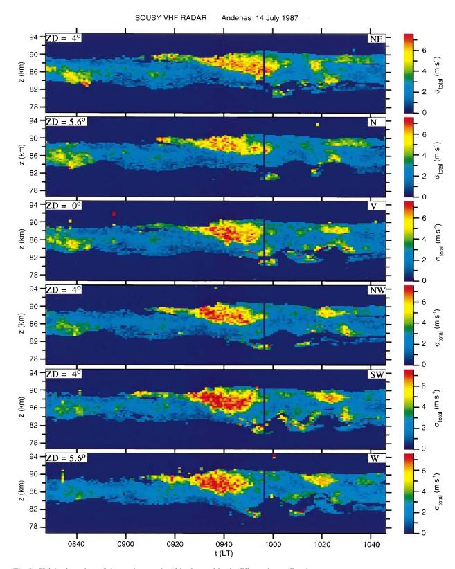
Fig. 2. Height-time plots of the total spectral width observed in six different beam directions
