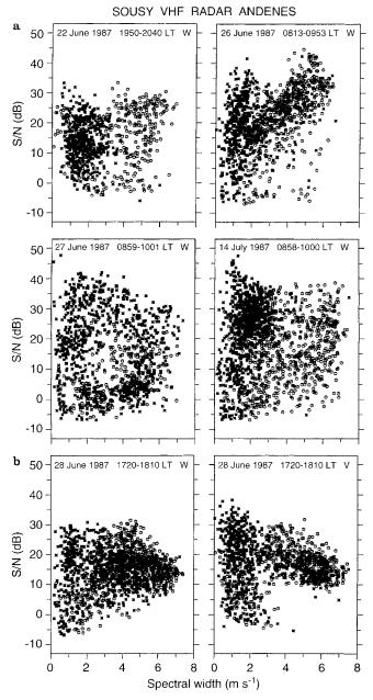
**Fig. 6a.** Scatter plots of  $\sigma_{turb}$  and S/N observed in the upper (*circles*) and lower (*asterisks*) sublayer of PMSE. **b** Scatter plots of  $\sigma_{turb}$  and S/N observed for antenna beams directed towards west (*left panel*) and vertically (*right panel*)
