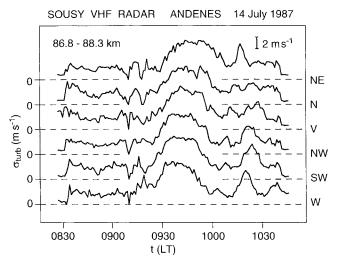
Fig. 7. Height integrated (86.2–88.3 km) time series of the turbulent component  $\sigma_{nurb}$  of the spectral width observed in all six beams
