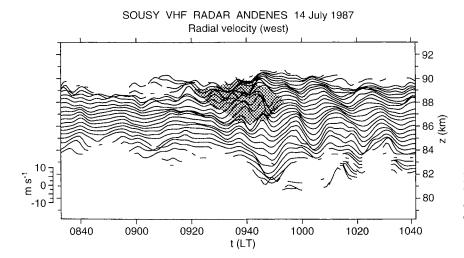
**Fig. 8.** Radial velocities versus time observed with a westward pointing beam. The *stippled area* denotes the extent of the structure of enhanced turbulence
