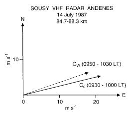
Fig. 10. Vector diagram of the phase trace velocities of the observed wave  $c_w$ , and the turbulent cells  $c_c$
