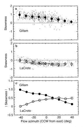
Fig. 6a-c. Dependence of the skewness versus the electron flow azimuth: a Scatterplot of skewness versus azimuth at the Gillam-Saskatoon link and the trend in this dependence (*large circles*); b the same has a, but for the LaCrete-Saskatoon link; c comparison of the trends on the G-S and L-S links
