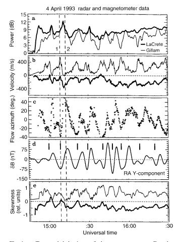
Fig. 4a–e. Temporal behaviour of the power **a**, mean Doppler velocity **b** and skewness **e** on the Gillam-Saskatoon (*thin line*) and LaCrete-Saskatoon (*thick line*) radio links during the period of pulsations. **c** Shows flow azimuth (CCW from the east) inferred from the G-S and L-S Doppler velocities. **d** Shows the rectified Y-component (east-west) of the Rabbit Lake magnetogram
