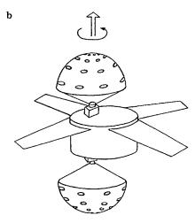
**Fig. 2. a** A schematic view of EU-1 analyzer. Sensor head consists of a toroidal electrostatic analyzer, channel electron multiplier MCP, followed by eight-sectored anode, electrostatic scanner consisting of central spherical electrode and grid-covered conic electrode, and sunshade baffle (collimator). **b** Sketch showing the viewing directions of two sensor heads of an instrument installed on rotating spacecraft. Sun direction is indicated by *arrow*
