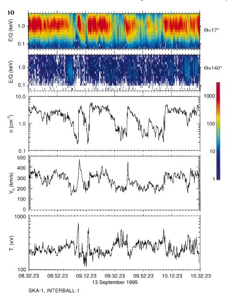
**Fig. 10.** The counting-rate spectra for two elevation cones of EU-1 during satellite pass in the vicinity of magnetopause on 13 September 1995 along with computed flow parameters, similar to format of Fig. 6
