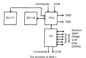
**Fig. 1.** The structure of SCA-1. It consists of two  $2\pi$  sensor heads EU-1/1 and EU-1/2, an onboard computer PVU, and controlling device UU-1
