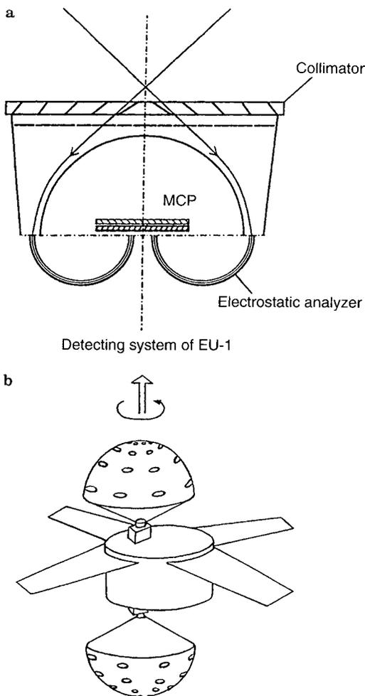
**Fig. 2.** a) A schematic view of EU-1 analyzer. Sensor head consists of a toroidal electrostatic analyzer, channel electron multiplier MCP, followed by eight-sectored anode, electrostatic scanner consisting of central spherical electrode and grid-covered conic electrode, and sunshade baffle (collimator). b) Sketch showing the viewing directions of two sensor heads of an instrument installed on rotating spacecraft. Sun direction is indicated by arrow
