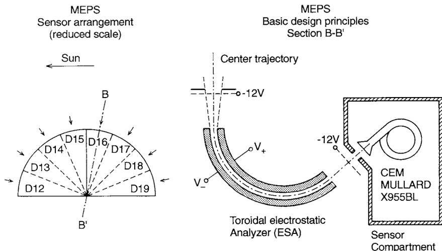
**Fig. 2.** Basic design principles of MEPS
