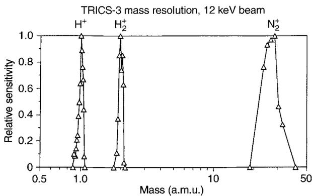
Fig. 6. Mass resolution of TRICS-3-Tail at 12 keV
