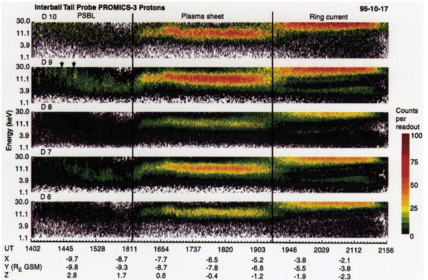
**Fig. 10.** Spectrogram obtained during a traversal of the magnetotail on 17 October 1995. The intensity scale is counts per readout, which is approximately proportional to the energy flux. The accumulation
