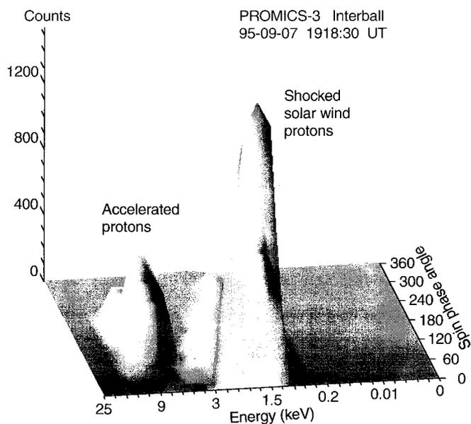
**Fig. 9.** Proton distribution measured in the dawnside magnetosheath at about  $30 R_E$  (GSM coordinates:  $-6.8, -23.2, 18.7$ ) on 7 September 1995 at 1918:30 UT. There were two distinct populations, shocked solar wind protons with a peak at about 1.5 keV and accelerated protons with a peak at about 8–9 keV
