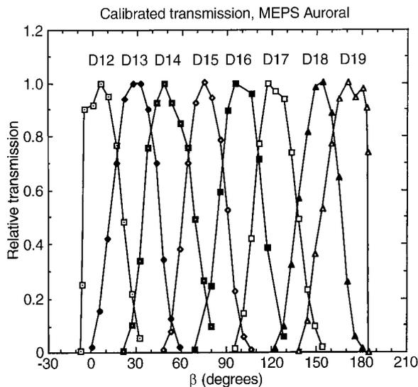
**Fig. 3.** Calibrated field of view of MEPS-Auroral
