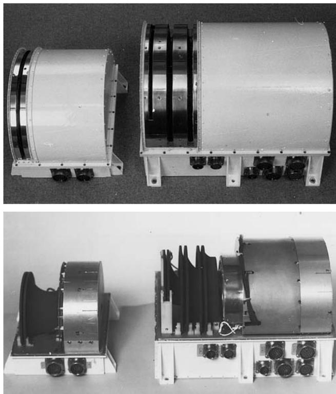
**Fig. 1.** PROMICS-3. The electron spectrometer MEPS is to the left and the positive ion spectrometer TRICS is to the right. The lower photograph shows the instrument with covers removed. Note the stacked design of the three TRICS toroidal electrostatic analyzers
