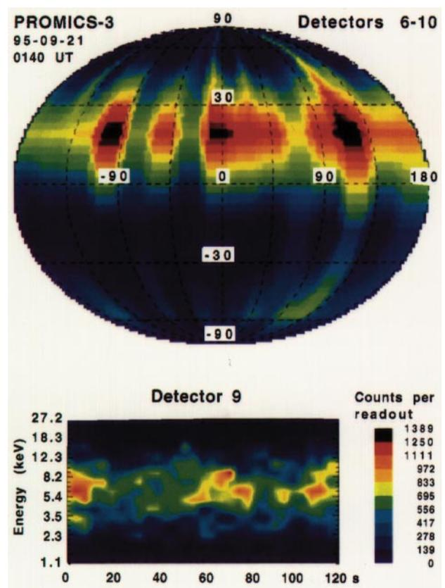
**Fig. 13.** Ring-shaped proton distribution with gyro bunching measured on 21 September at 0140 UT in the dawnside plasma sheet (SM coordinates:  $-3.5, -13.1, -2.8$ ). The *upper part* shows the total number of protons in the energy range 1–30 keV as a function of direction of incidence. The *lower part* shows a spectrogram measured by D9 during one spin. This spectrogram constitutes the contribution from D9 to the *upper part* of the figure. The *scale* applies only to the *lower part*
