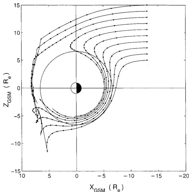
**Fig. 12.** Drift trajectories of protons with an initial energy of 0.5 keV and pitch angle  $45^\circ$  in a dawn-dusk electric field of 0.1 mV per meter. Such particles may be the source of the 3 keV population occurring simultaneously with the ring current in Fig. 10
