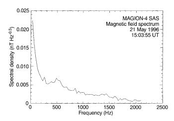
Fig. 5. The spectrum of the magnetic-field ( $B_x$ -component) fluctuations taken during the magnetopause crossing
