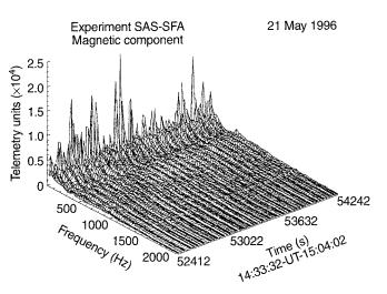
Fig. 4. The same as in Fig. 2 for the magnetopause crossing on 21 May. The sharp enhancement at the lowest frequency can be seen at 14:39, 14:45 and 14:58 UT. The co-ordinates of the satellite were  $r = 10.4-11.7 \text{ R}_{\text{E}}$ , Mlat = 62–57°, MLT $\approx$ 12
