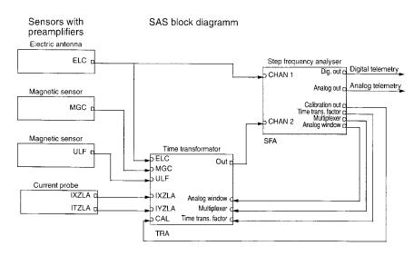
perpendicular to it. The sensitivity of these measurements is  $3 \cdot 10^{-5}$  nT Hz<sup>-1/2</sup> at 100 Hz. The output signal of the detectors is processed by the step-frequency spectrum analyser: SAS.
